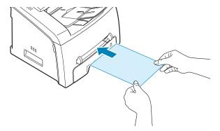
For envelopes, load a sheet with the flap side face down and with the stamp area on the top left side.
